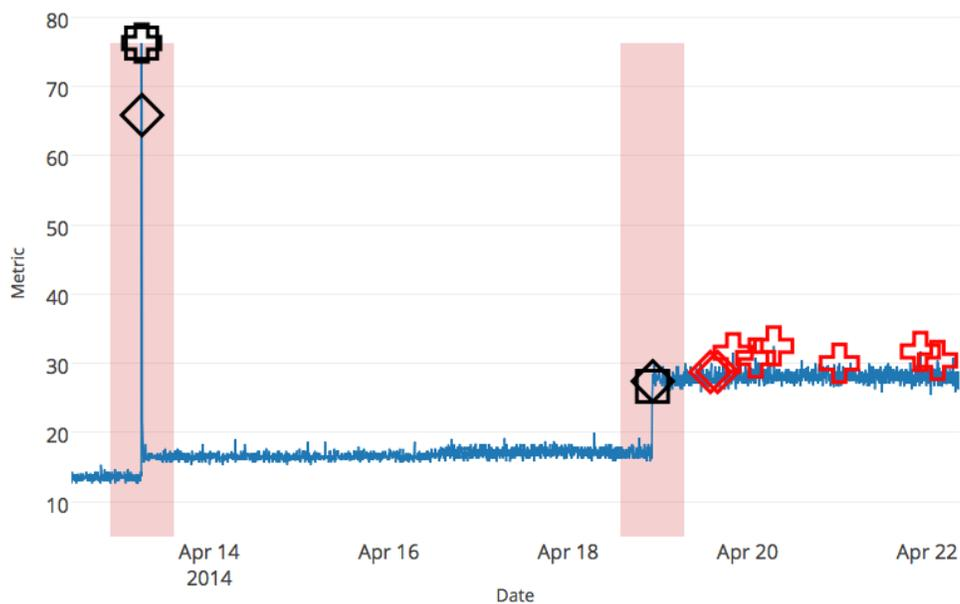
Figure 1. Detection results for anomalies on a production server based on CPU usage. A black shape indicates the first true positive detected. A red shape indicates a false positive. The red shaded regions denote the anomaly windows.
